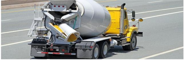
Ready-mixed concrete is concrete that is manufactured in a batch plant, according to a set engineered mix design. Ready-mixed concrete is normally delivered in two ways. First is the barrel truck or in-transit mixer. This type of truck delivers concrete in a plastic state to the site.
